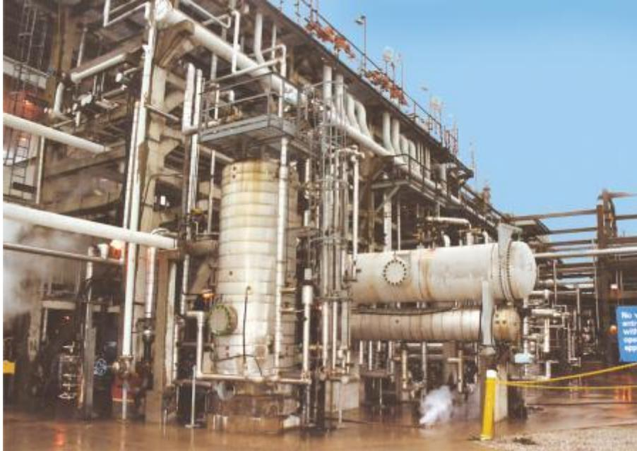
Heavy raw materials are generally difficult to process by FCC or reforming, but can be converted by hydrocracking. The feedstock is cracked by catalytic cracking in the presence of hydrogen, which produces a mixture of gasoline and distillate. There are about a dozen different hydrocracking processes in use.
